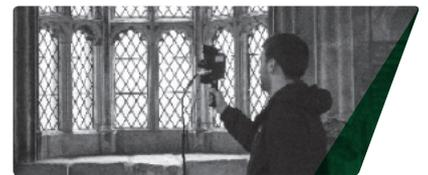
**Rapid scanning time** – within minutes anyone can be operating the ZEB-REVO, and our intelligent software (which uses the most established and robust SLAM mapping algorithm in the industry) can map a 3-storey building in just 30 minutes to an accuracy level of  $\pm 15\text{mm}$ , or map a 10,000 m<sup>2</sup> (105,000 sq. ft.) depot in under an hour. Walk through your target survey environment to record more than 43,000 measurement pts/sec, and from scan to full 3D BIM model in under an hour!
