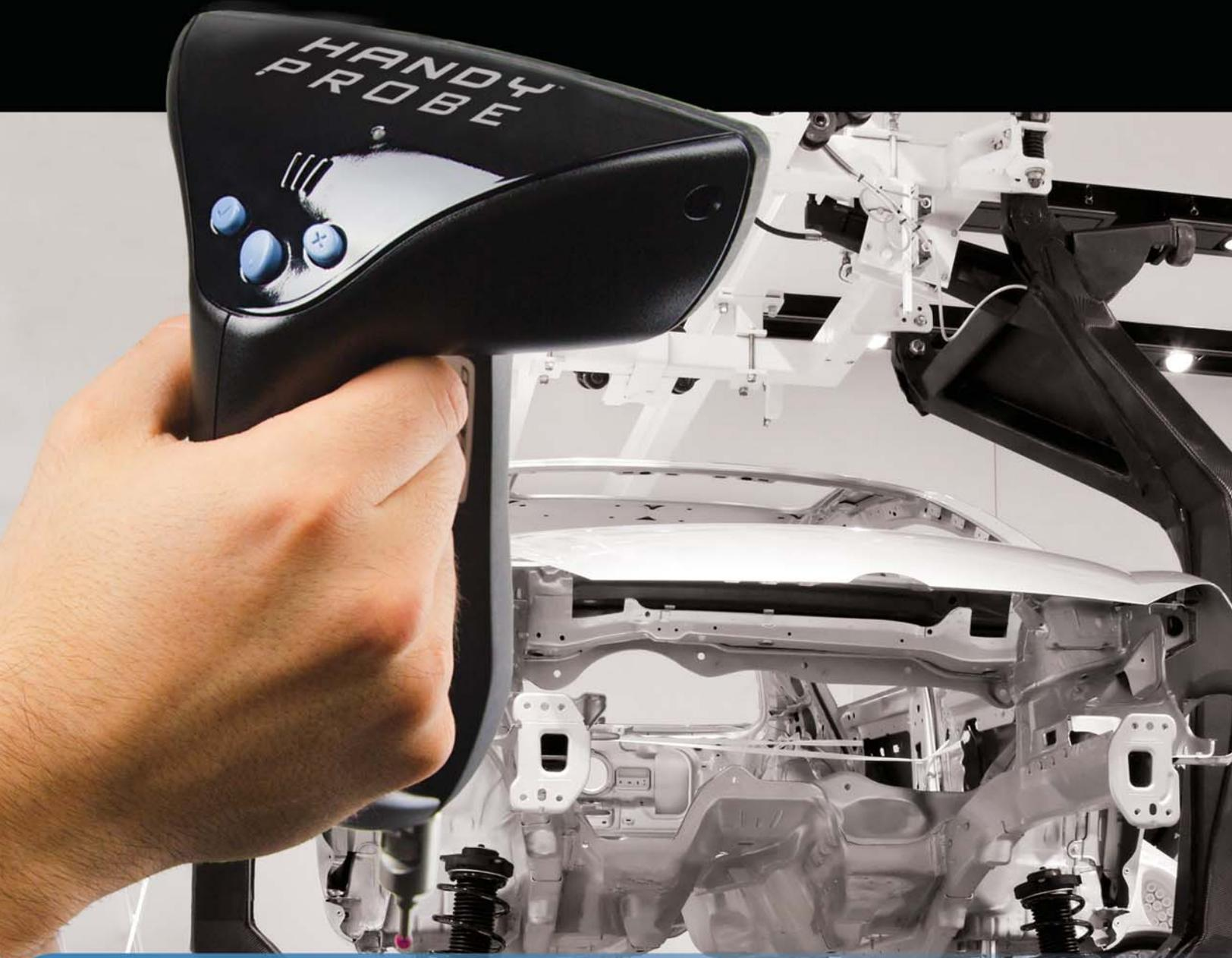
The HandyPROBE™ arm-free portable probing system and the C-Track™ dual-camera sensor form a unique duo that generates high-accuracy measurements with an accuracy of up to **22 µm** and also increases the reliability and speed of the measurement process. This portable CMM was designed and optimized to operate in “real-life” shop floor conditions.
